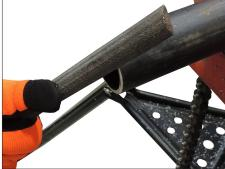
**3.** Using a flat-mill file, remove all sharp edges and burrs while creating the rounded-over pipe end detail that is shown on page 1. Once completed, the pipe end shall not contain sharp edges or burrs (refer to photo of good pipe below). For additional clarification, scan the QR code below to access the pipe preparation video.
