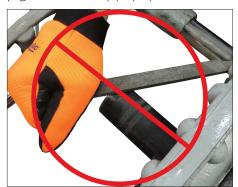
DO NOT hold the file at an angle, as shown. This will push burrs toward the pipe end, resulting in an unacceptable condition. For additional clarification, scan the QR code on the following page to access the pipe preparation video.
