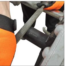
**3.** Turn power drive on. Using a flat-mill file, remove all sharp edges and burrs while creating the rounded-over pipe end detail that is shown on page 1. **NOTE:** The file shall remain perpendicular to the pipe during this operation. Once completed, the pipe end shall not contain sharp edges or burrs (refer to photo of good pipe end below). For additional clarification, scan the QR code on the following page to access the pipe preparation video.
