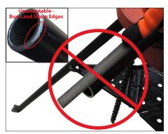
DO NOT file toward the pipe end. This will push burrs toward the pipe end, resulting in an unacceptable condition. For additional clarification, scan the QR code below to access the pipe preparation video.
