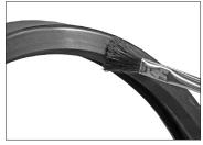
2b. IF ANY CONDITIONS LISTED IN THE FOLLOWING NOTICE ARE MET, APPLY A THIN COAT OF A COMPATIBLE LUBRICANT ONLY TO THE GASKET SEALING LIPS: For EPDM gaskets, use Victaulic Lubricant or an EPDMcompatible lubricant.
