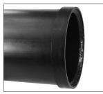
1. CHECK SHOULDERED PIPE ENDS: The outside surface of the shouldered pipe end shall be generally free from indentations and projections to ensure a leaktight seal. All oil, grease, loose paint, dirt, and cutting particles shall be removed.
