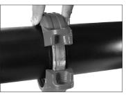
**5. INSTALL HOUSINGS:** Install the housings over the gasket. Verify that the housings' keys engage the shouldered pipe ends.
