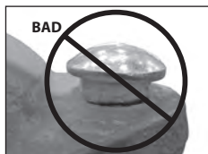
OVAL NECK OF BOLT NOT SEATED PROPERLY
