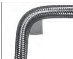
2-INCH/51-MM MINIMUM BEND RADIUS
