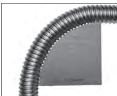
4-INCH/102-MM MINIMUM BEND RADIUS
