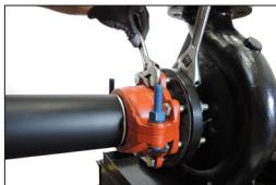
**9. TIGHTEN FLANGE NUTS:** Tighten all nuts evenly in a crossing pattern, in accordance with a regular flange assembly. Continue to tighten all nuts until the standard, flanged joint torque requirement is reached. Refer to the "Style 904 Helpful Information" table for typical and maximum torque values.
