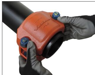
**6a. INSTALL COUPLING:** Assemble the joint by inserting the marked HDPE pipe ends into each opening of the coupling. The first HDPE pipe end must be inserted through the coupling until the pipe end is visible from both sides of the coupling.
