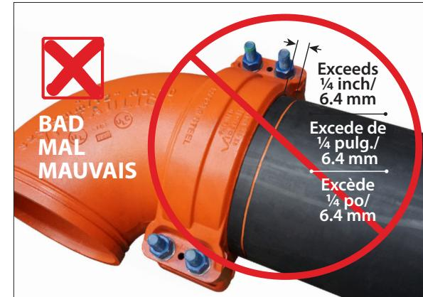
**7. INSPECT BOLT PADS:** Before pressurizing the system, inspect the bolt pads at each joint to ensure that proper assembly is achieved.
