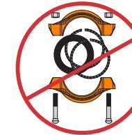
**1a. DO NOT DISASSEMBLE THE COUPLING:** Style 907 Couplings are designed so that the installer does not need to remove the bolts and nuts for installation. This design facilitates installation by allowing the installer to directly insert mating component ends into the coupling.
