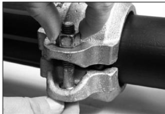
8. Insert the bolts. Thread a nut onto each bolt finger-tight. **NOTE:** Make sure the oval neck of each bolt seats properly in the bolt holes.
