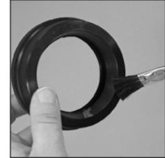
4. Check the gasket to make sure it is suitable for the intended service. The color code identifies the gasket grade. Lubricate the gasket in accordance with the "Lubricant Compatibility for Gaskets" table. **DO NOT use Victaulic lubricant on HDPE pipe.** Always consult with the pipe manufacturer for lubricant compatibility requirements.
