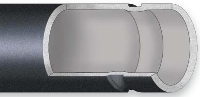
Roll groove shown on Schedule 40 steel pipe. The small dimple created on interior pipe wall does not significantly hinder pressure or flow.
