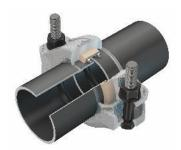
Pipe is simply joined by positioning the coupling seal and housing segments on the pipe ends and tightening the bolts and nuts to the specified torque requirement. Installation is completed up to five times faster than other joining methods.
