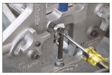
**2.** Using a flat-head screwdriver, rotate the "A" adjustment screw counterclockwise to adjust the groove location.
