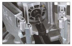
**7.** Use the provided 5/4-inch T-Handle hex key to loosen the set screw. This will allow the depth stop to move.
