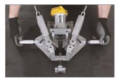
**2.** While supporting the tool on a level surface, screw the handles into the sides of the tool until hand-tight. Do not overtighten.
