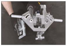
**4.** The 2–4 inch arms must be mounted on the tool in a specific orientation. Match the "A" or "B" etched on the arm with the corresponding letter on the tool body, then insert the arms into the tool body so that the matching letters face each other.
