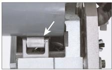
**5.** Put the toggle clamps in the engaged position, then twist until the OD and ID rollers are touching the pipe. Do not over-tighten.
