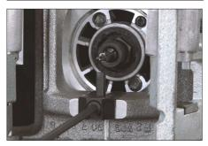
**9b.** To set the depth stop, use the provided  $\frac{3}{6}$ -inch T-Handle hex key to turn the adjustment screw, which will move the depth stop back and forth. Align the tip of the cutting bit with the line on the alignment block that matches the pipe size to be grooved.
