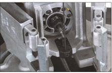
**7.** Use the provided  $\frac{1}{64}$ -inch T-handle hex key to loosen the set screw. This will allow the depth stop to move.
