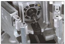
**6.** Verify that the cutter bit is inserted deeply enough for the etched line to be partially or fully covered by the collet.
