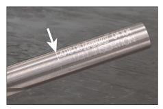
**2b.** Take note of the line etched on the base of the bit. This marks the minimum depth of insertion when installing the bit into the tool.
