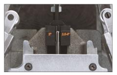
**9c.** Verify the alignment of the tip of the cutter bit with the appropriate line on the alignment block. The cutter bit pictured above is set for 2.5 to 4-inch pipe.
