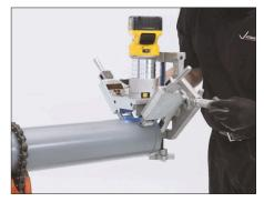
**5.** Grasp both handles and slowly push the tool through one complete clockwise rotation. At the end of the rotation, push the tool slightly past vertical to ensure that the groove is complete.
