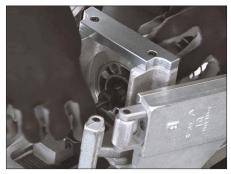
**4.** Insert the 6–12 inch cutter bit into the collet to just past the minimum insertion depth.
