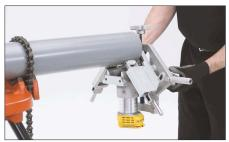
**6.** Tighten the arm locking knobs to hand-tight. Do not over-tighten.
