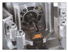
8. Align the notch on the back of the alignment block with the depth stop behind the bit. Slide the alignment block over the depth stop until fully seated.
