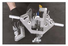
**4.** The 6–12 inch arms are interchangeable and may be mounted on the tool in either orientation. Insert the arms into the body of the tool.
