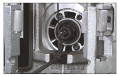
11. Hold the  $\frac{3}{6}$ -inch hex key in the adjustment screw to stop any movement and tighten the set screw to lock the depth stop in place.
