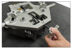
**8.** Using the motor carriage adjustment knob, verify that the bit is positioned high enough to clear the pipe OD when mounting the tool. Rotate the knob counterclockwise to raise the bit and clockwise to lower the bit.
