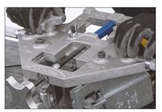
**3.** Loosen the arm locking knobs to allow room to mount the tool onto the pipe.
