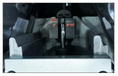
**9a.** Select the appropriate cutter bit location by matching the pipe size to the corresponding line on the alignment block.
