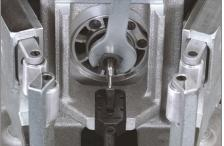
**5.** While pressing the spindle lock button, use the  $\frac{1}{16}$ -inch wrench to tighten the collet. Do not overtighten.
