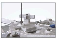
**7.** Tighten the shoulder bolts using the provided hex key.
