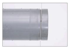
**11.** Once the groove is clean, check the groove diameter ("C" dimension). A pipe diameter cable, supplied with the tool, is the recommended method for checking the "C" dimension.
