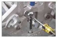
**2.** Using a flat-head screwdriver, rotate the "A" adjustment screw clockwise to adjust the groove location.
