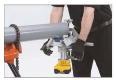
**8.** Put the toggle clamps in the disengaged position.
