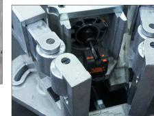
**8.** Align the notch on the back of the alignment block with the depth stop behind the bit. Slide the alignment block over the depth stop until fully seated.
