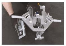
**3.** Pull the 2–4 inch arms straight out from the body of the tool. When not in use, store the arms in the provided tool box.
