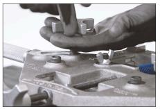
1. Unscrew and remove the arm locking knobs.
