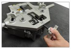
**2.** Using the motor carriage adjustment knob, verify that the bit is positioned high enough to clear the pipe OD when mounting the tool. Rotate the knob counterclockwise to raise the bit and clockwise to lower the bit.
