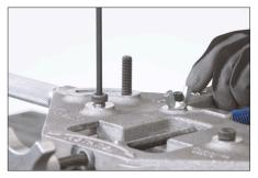
**2.** Loosen and remove the shoulder bolts using the provided hex.
