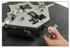
**8.** Using the motor carriage adjustment knob, verify that the bit is positioned high enough to clear the pipe OD when mounting the tool. Rotate the knob counterclockwise to raise the bit and clockwise to lower the bit.
