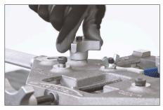
**6.** Replace the arm locking knobs and screw down until the arms are secure against the body of the tool.
