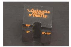
**1.** Retrieve the 6" THRU 12" alignment block. Alignment blocks are etched with the pipe size in inches.
