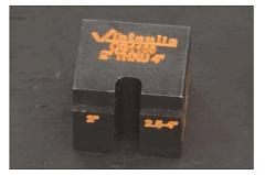
**1.** Retrieve the 2" THRU 4" alignment block. Alignment blocks are etched with the pipe size in inches.
