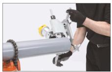
**7a.** Push the tool through one complete clockwise rotation to check for obstructions and to allow the tool to track onto the pipe. Verify that the tool moves freely throughout the entire rotation.
