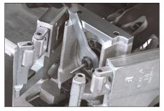
**3.** While pressing the spindle lock button, use the  $\frac{1}{16}$ -inch wrench to loosen the collet. Remove the 6–12 inch bit.
