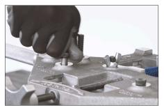
**5.** Replace and tighten the shoulder bolts to finger-tight.
