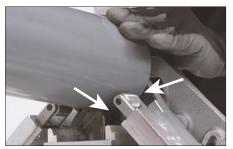
**7b.** If the tool tracks properly and the pipe stops retain contact with the pipe end, the arm setting is correct.
