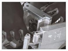
**4.** Insert the 2–4 inch cutter bit into the collet to just past the minimum insertion depth.
