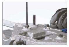
**2.** Loosen and remove the shoulder bolts using the provided hex key.
