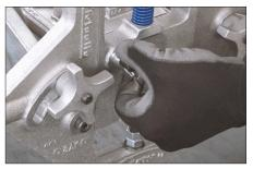
**1.** Loosen the wing nut on the "A" adjustment screw, located on the front of the tool.
