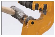
**3.** Tap the cutting wheel shaft into the tool body to secure the new cutting wheel.
