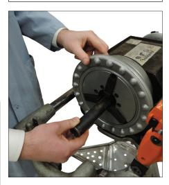
**5.** Insert the pipe into the power drive and tighten the chuck at the proper pipe length.
