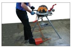
**3a.** Depress the safety foot switch to start the power drive.
