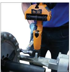
**3.** Using a hammer or mallet, tap the hinge pin into the bracket slot until it is secure. Do not force the hinge pin farther into the slot than is necessary to secure the PC3110.
