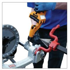
**1.** Place the PC3110 over the bracket on the carriage assembly.
