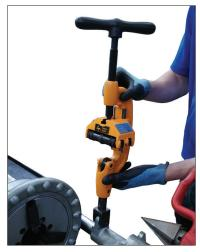
**1.** To turn the PC3110 for carriage storage, lift the body of the PC3110 away from the shaft.
