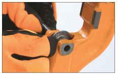
2. Install the new cutting wheel and insert the cutting wheel shaft (use the new cutting wheel shaft if the cutting wheel kit was ordered).
