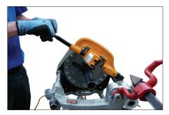
**4.** Using the handle, lift the PC3110 back to its storage position.
