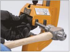
**3.** Install the new chamfering roll at the front of the tool body, as shown, then insert the new chamfering roll shaft from the kit. Tap the new chamfering roll shaft into the tool body to secure the new chamfering roll.
