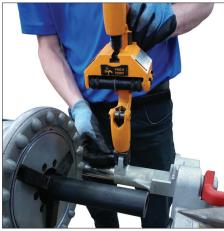
2. Insert the hinge pin into the bracket slot.
