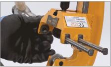
1. Using a hammer and punch, tap each roll shaft out of the tool body. Remove and discard each worn-out roll and roll shaft.
