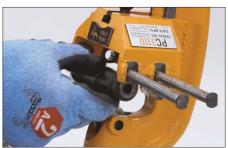
**2.** Install the new flattening roll at the back of the tool body, as shown, then insert the new flattening roll shaft from the kit. Tap the new flattening roll shaft into the tool body to secure the new flattening roll.
