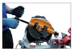
**1.** Using the handle, bring the PC3110 down over the pipe end.
