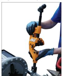
**2.** Twist the body of the PC3110 90 degrees counterclockwise so that the knurled rolls face the front of the carriage, then lower the body of the PC3110 back down towards the shaft.
