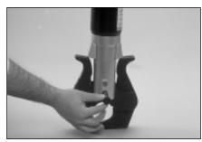
**3.** Align Pressfit Tool over the jaws, engaging the tool into the jaws being certain to check the jaw alignment. When in position push the locking pin into the tool until it clicks into the fully locked position.
