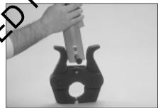
**2.** Place the proper size press jaw on a table or the floor. Slide the locking pin to its fully open position.
