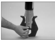
**3.** While holding the tool vertically, slide locking pin to its fully open position.
