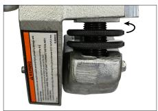
**3a.** Turn the upper depth stop collar (closest to the trunnion) until the distance between the collar and the top of the trunnion is equal to the groove depth gauge thickness.
