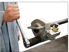
5. A ratchet with  $1\,\%$ " socket (not supplied) may be used in place of the crank to operate the tool in low clearance conditions.
