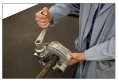
**3.** Advance the feed by turning the feed nut clockwise by ½ turn.
