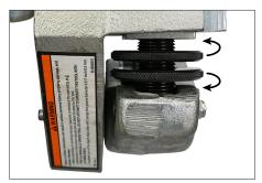
**1.** Unlock the depth stop collars by turning them in opposite directions until they are separated.
