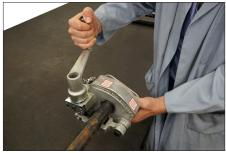
**2.** Turn the feed nut counterclockwise to retract the upper roll arm to the full open position.
