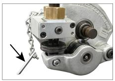
**2.** Locate the groove depth gauge attached to the tool.
