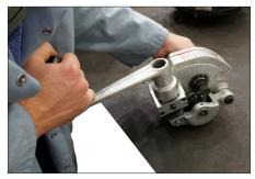
1. Using the crank, retract the upper roll arm fully by turning the feed nut counterclockwise.
