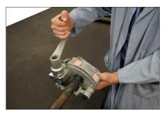
**6.** Advance the feed by turning the feed nut clockwise by ½ turn. Crank the tool another full turn around the pipe.
