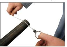
**4.** After dismounting the tool from the pipe, check the groove diameter to ensure that the groove meets specification.
