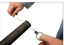
5. After a trial groove is prepared and the tool is removed from the pipe, carefully check the groove diameter ("C" dimension), as charted in the "Roll Groove Specifications" section. The "C" dimension is best checked with the provided Go/No-Go cable. It also may be checked with a pi tape, vernier caliper, or narrow land micrometer at two locations, 90° apart, around the groove. The average reading must equal the required groove diameter specification.
