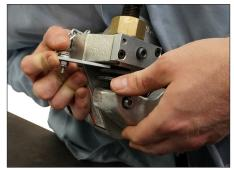
**3c.** Turn the lower depth stop collar until both depth stop collars are locked firmly against one another, maintaining the gap that was set with the groove depth gauge.
