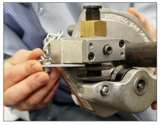
**3b.** Use the groove depth gauge like a feeler gauge to position the upper depth stop collar.
