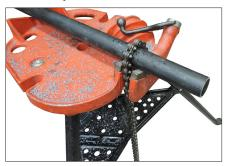
**3.** Secure a length of pipe in the pipe vise. Pipe position and pipe vise anchoring must be capable of handling the weight of the tool (17 pounds/8 kilograms), plus the manual effort required to operate the tool (approximately 20 ft-lbs/27 N•m of torque). Position the pipe to overhang the pipe vise by approximately 5–12 inches/125–300 mm, as shown, so that the tool can rotate freely around the pipe.
