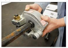
**2.** With the drive nut down, insert the lower roll into the pipe end. Push the tool onto the pipe until the pipe end stop rests against the pipe end.
