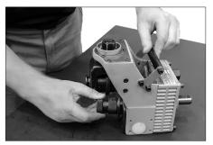
**3.** Grasp the drive shaft with one hand, then use the other hand to pull the lower roll straight off of the tool.
