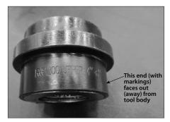
**1.** Verify the appropriate roll size by checking the marking on the edge of the roll.
