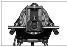
**9.** Ensure that the tool is stable and is centered on the power drive support arms.
