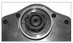
**1.** Each rotation line around the groove diameter adjustment nut signifies 0.016 inches/0.4 mm of groove diameter adjustment.
