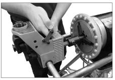
**6.** Insert the tool drive shaft into the power drive adapter until the tool body meets the adapter.
