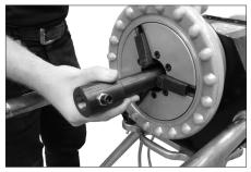
**5.** Insert the power drive adapter into the power drive until the adapter collar meets the drive collet.
