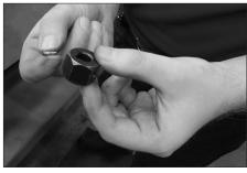
Remove the shear pin using the shear pin punch and replace with an intact shear pin. If all provided shear pins have been used, contact Victaulic to order replacements.
