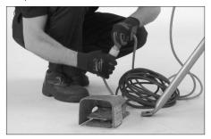
**3.** Plug the power drive cord into the provided safety foot switch, as shown above. Refer to the power drive manufacturer's operating manual for additional information.
