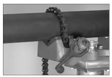
**3.** Secure a length of pipe in the pipe vise. Pipe position and pipe vise anchoring must be capable of handling the weight of the tool (27.7 pounds/12.6 kilograms), plus the manual effort required to operate the tool (approximately 75 ft-lbs/101.7 N•m of torque).
