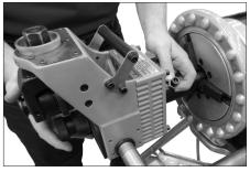
**8.** Tighten the shoulder nut until hand-tight. Do not overtighten.
