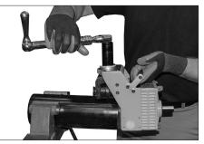
**4.** Mount the tool on the pipe, then turn the groove diameter adjustment nut clockwise to lower the upper roll until the tool rests snugly on the pipe.
