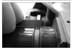
**5.** While supporting the tool, loosen the groove diameter adjustment nut and remove the tool from the pipe.
