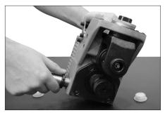
**4.** Screw the support arms into the ports until hand-tight. Do not overtighten.
