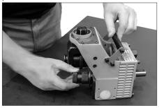
**5.** Grasp the tool with one hand, then use the other hand to push the lower roll into the tool.
