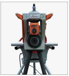
**13.** Ensure that the tool is stable, centered, and level on the power drive support arms.
