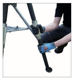
**12.** Twist the tool legs until the feet rest flat against the ground.
