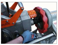
11. Using the hex key provided, tighten the socket cap screw until hand-tight. Then, tighten the locking nut until hand-tight. Do not overtighten.
