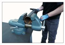
**3.** Secure a length of pipe in the pipe vise. Pipe position and pipe vise anchoring must be capable of supporting the weight of the tool (95.5 pounds/43.3 kilograms), the weight of the pipe, and the force generated during operation of the tool.
