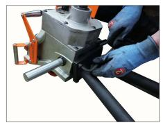
**8.** Using the hex key provided, tighten the socket cap screws to secure the leg assembly to the base of the tool head. Do not overtighten.
