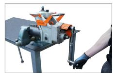
**2b.** Using the provided handle, turn one of the manual drive nuts to begin grooving.
