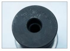
**1.** Verify the appropriate roll size by checking the marking on the front of the roll.
