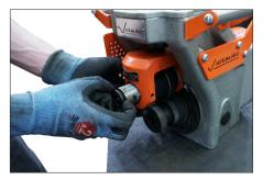
**3.** Remove the upper roll shaft by drawing it out from the slide assembly.
