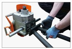
**6.** Align the leg assembly with the base of the tool head. Proper orientation will have the legs angled towards the front of the tool body.
