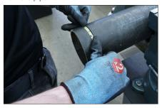
**8.** Carefully check the groove diameter of the pipe ("C" dimension) with the provided Go/No-Go Groove Diameter Tape.
