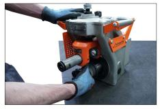
**3.** Grasp the tool with one hand, then use the other hand to pull the lower roll out of the tool.
