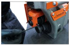
**2.** Using the hex key provided, loosen the set screw on the side of the slide assembly. It is not necessary to fully remove the set screw.
