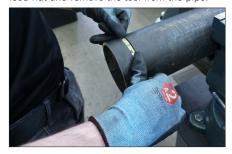
**6.** Carefully check the groove diameter of the pipe ("C" dimension) with the provided Go/No-Go Groove Diameter Tape.
