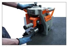
**1.** Replace the lower roll with the alternate size provided.
