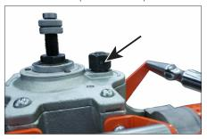
1. To access the shear pin in the depth feed nut, turn the depth feed nut sideways to allow room for the shear pin punch.
