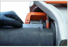
**5.** While supporting the tool, loosen the depth feed nut and remove the tool from the pipe.
