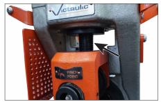
2. Once per week, use EP2 lithium grease to lubricate the groove diameter adjustment screw. To make room for lubrication, move the groove diameter adjustment nuts to the top of the threaded rod. Remove the lower roll, then lower the slide assembly until the groove diameter adjustment nuts bottom out on the tool head.
