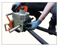
7. Insert the provided socket cap screws.
