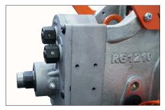
**2a.** The upper left manual drive nut is high speed/low torque for smaller diameter pipe. The lower right manual drive nut is low speed/high torque for larger diameter pipe.
