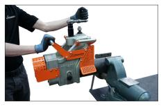
**4.** Mount the tool on the pipe, then turn the depth feed nut clockwise to lower the upper roll until the tool rests snugly on the pipe. Move the groove diameter adjustment nuts to the top of the threaded rod so as not to interfere with the setup groove.
