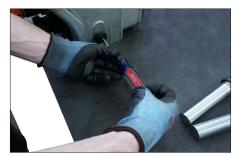
**3.** Using a flat-head screwdriver, remove the caps on the support arm ports.
