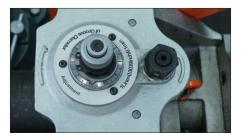
1. Each rotation line around the groove diameter adjustment nut signifies 0.0039 inches/0.1 mm of groove diameter adjustment.
