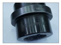
1. Verify the appropriate roll size by checking the marking on the edge of the roll.
