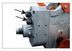
**2b.** Turn the manual drive nuts sideways to allow room for the shear pin punch.
