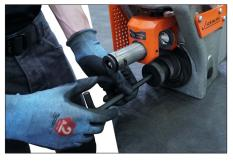
**3.** Using the hex key provided, reinstall the lower roll retaining stud.
