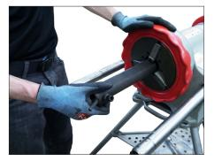
**9.** Insert the power drive adapter into the power drive until the adapter collar meets the drive collet.
