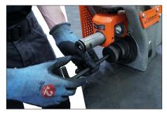
**2.** Using the hex key provided, remove the lower roll retaining stud.
