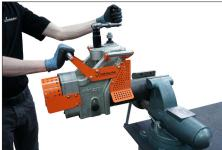
**3.** Alternate turning the depth feed nut with turning the manual drive nut. Do NOT turn the depth feed nut more than 0.0039 inches/0.1 mm (one line) per rotation.
