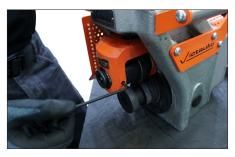
1. Replace the upper roll and upper roll shaft into the slide assembly. To confirm proper installation, verify that the part code stamp on the upper roll faces the operator. Also verify that the upper roll groove feature aligns with the lower roll pocket. Tighten the set screw until hand-tight.
