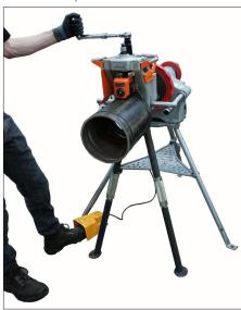
**5.** Press the safety foot switch to begin grooving. Do NOT turn the depth feed nut more than 0.0039 inches/0.1 mm (one line) per rotation.
