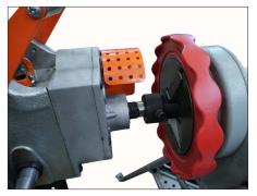
10. Insert the tool drive shaft into the power drive adapter until the tool body meets the adapter. NOTE: A hoist eye has been provided to allow the use of a lifting device when mounting the tool.
