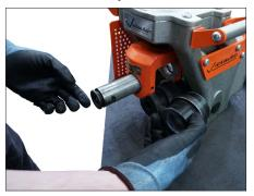
**4.** Remove the upper roll from the slide assembly.
