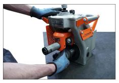
**2.** Grasp the tool with one hand, then use the other hand to push the lower roll into the tool.
