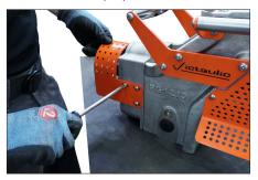
**2a.** To access the shear pins in the manual drive nuts, unscrew the safety guard and set aside.
