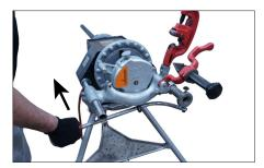
**2.** Using the carriage lever, push the grooving head fully over the pipe end.
