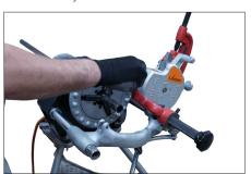
**7.** Use the handle to lift the reamer back to its storage position.
