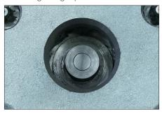
Periodically inspect the pipe insertion area on the front of the grooving head. If any debris is visible inside the grooving cup, clear away the material with a wire brush.
