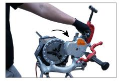
**6.** Using the handle, lift the grooving head back to its storage position.
