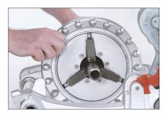
**5.** Insert the pipe into the power drive and tighten the chuck at the proper pipe length.
