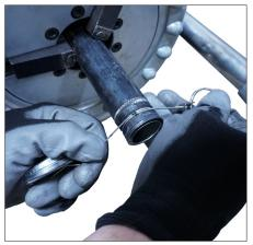
Carefully check the groove diameter ("C" dimension) using the provided groove confirmation cable. Refer to the "Roll Groove Specifications" section.
