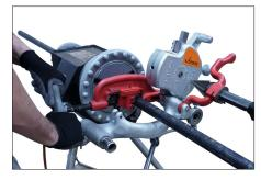
2. Depress the safety foot switch to start the power drive, then turn the handle of the cutter in a steady motion until the pipe end is cut and falls off. Remove foot from the safety foot switch.
