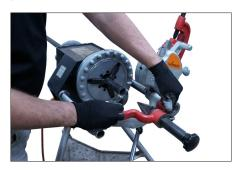
**5.** Push the release lever open and slide the reamer forward until it locks into the extended position.
