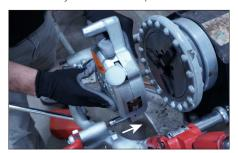
1. With the grooving head up in the storage position, grasp the head with both hands and pull it towards the power drive to remove it from the carriage assembly.
