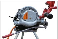
**1.** Using the handle, bring the grooving head down to rest on the carriage assembly.
