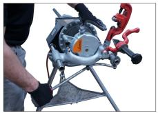
**4.** Maintain grip on the carriage lever to keep the tool in position during grooving. Depress the safety foot switch to start the power drive, then press and release the actuator. **NOTE:** Keep all other objects away from the tool during the grooving process.
