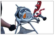
**5.** Hold the grooving position until the Ready-to-Groove Indicator stops rotating, signaling that the groove is complete. Remove foot from the safety foot switch and use the carriage lever to pull the grooving head free from the pipe end.
