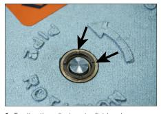
1. To align the rolls, insert a flat-head screwdriver into the notches that bisect the Ready-to-Groove Indicator. Twist the screwdriver in either direction until the indicator pops into the locked position, so that it no longer protrudes from the cover.
