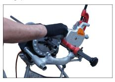
**4.** Using the handle, bring the reamer down to the pipe end.
