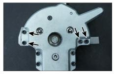
**2.** Place the grooving head on a flat surface. Remove the four screws holding the two adapters in place, then remove the adapters.
