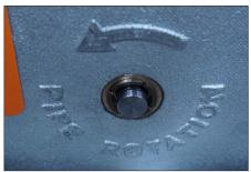
**3.** When the grooving head is pushed fully over the pipe end, verify that the Ready-to-Groove Indicator on the rear face of the grooving head pops out. This provides visual confirmation that the tool is unlocked and ready for grooving. If the indicator is not protruding, the tool is still locked and will not operate.
