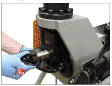
**2.** While supporting the upper roll, insert the upper shaft into the slide and upper roll.
