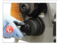
**3.** Remove the lower roll retaining nut from the lower roll arbor. Store in a safe location for future use.
