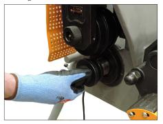
1. Insert the desired lower roll into the lower roll bore until it contacts the tool body.
