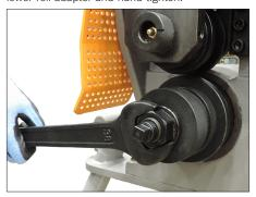
**6**. Tighten the lower roll retaining nut with a 38-mm wrench (included) to retain the lower roll on the lower roll adapter.
