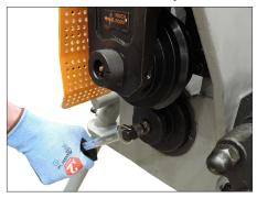
**2.** Tighten the lower roll by turning it counterclockwise with the 14-mm wrench (included).
