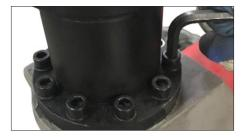
2. Remove the bolts supporting the cylinder.
