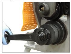
**2.** Loosen the lower roll retaining nut with the 38-mm wrench (included).
