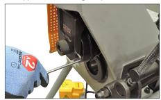
**2.** Loosen the upper shaft retaining screw with the 5-mm hex key (included). DO NOT completely remove this screw.
