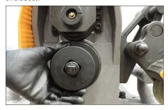
**3.** Install the desired size lower roll onto the lower roll adapter with the marked side facing outward.
