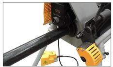
**3.** Insert a piece of pipe of the correct size and wall thickness onto the lower roll.
