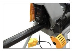
**5.** Insert a piece of pipe of the correct size and wall thickness onto the lower roll.
