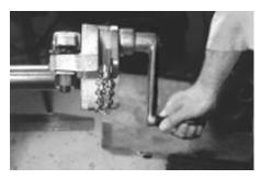
**4.** Place the crank onto the drive hex. Crank the drive hex either clockwise or counterclockwise until the tool travels one full turn around the pipe.
