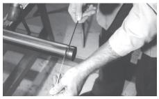
**4.** After dismounting the tool from the pipe, check the groove diameter to ensure that the groove meets specification.
