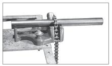
3. Secure a length of pipe/tubing in the pipe vise. Pipe/tubing position and pipe vise anchoring must be capable of handling the weight of the tool (17 pounds/8 kilograms), plus the manual effort required to operate the tool (approximately 20 ft-lbs/27 Nom of torque). Position the pipe/tubing to overhang the pipe vise by approximately 5-12 inches/125-300 mm, as shown, so that the tool can rotate freely.
