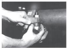
3. Turn the depth stop collar, closest to the trunnion, until the distance between the collar and the top of the trunnion is equal to the groove depth gauge thickness. Use the groove depth gauge like a feeler gauge. Turn the second collar until both are locked firmly against one another, maintaining the gap set with the groove depth gauge.
