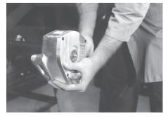
With the drive nut down, insert the lower roll into the pipe end. Push the tool onto the pipe until the pipe end stop rests against the pipe end.
