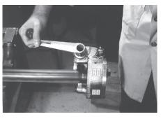
**6.** Advance the feed by cranking the feed nut per the "Feed Rates" section. Crank the tool another full turn around the pipe.
