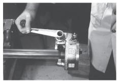
**3.** Using the crank, advance rolls together by turning the feed nut clockwise. Continue advancing until the grooving rolls are in light, but firm, contact with the pipe.
