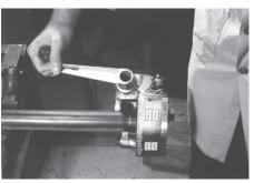
3. Advance the feed by turning the feed nut clockwise by the amount shown in the "Feed Rates" section. Feed rates for the VE12 vary depending on material and wall thickness.
