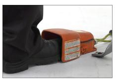
**4.** Depress the safety foot switch. Verify that the lower roll rotates away from the operator when viewed from the front of the tool. (See Figure 2 on page 21 for more information.) If the lower roll rotates toward the operator, reverse the rotation collar as outlined in step 7. Remove foot from the safety foot switch.
