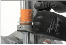
**5.** Back off the groove diameter stop by loosening the travel stop adjuster.
