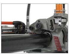
**7.** Insert a length of pipe that is the correct size and thickness onto the lower roll.
