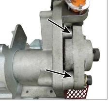
**3.** Apply grease to all locations where the roll arm slides against the tool body.
