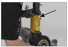
**5a.** Locate the rotation collar at the base of the Rems drive body.
