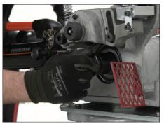
**4.** Install the lower roll/main shaft into the tool head. While maintaining a grip on the knurled end (lower roll) of the main shaft, ensure that the flats on the drive end of the main shaft align with the flats in the power drive adapter.
