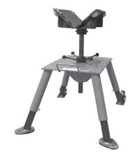
The Victaulic VAPS112 is a portable, adjustable, roller-type pipe stand that contains four legs for additional stability. Ball transfer rollers, adjustable for 2-12-inch/60.3-323.9-mm pipe, and the "V" rest for 34-11/2-inch/ 26.9-48.3-mm pipe, accommodate linear and rotational movement. The turnstile design permits ease of grooving for both pipe ends. Contact Victaulic for details
