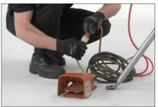
**9.** Plug the Ridgid 700 power drive cord into the safety foot switch, as shown above. Plug the safety foot switch cord into a grounded electrical outlet. Refer to the power drive manufacturer's operating manual for additional information.
