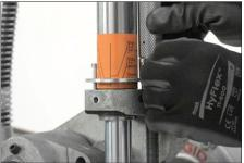
**14.** When the depth stop indicator top plate is properly aligned, tighten the travel stop adjuster to lock in the setting.
