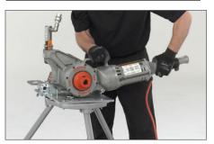
1. Place the Ridgid 700 power drive on the back of the stand assembly. Align the tapped hole in the Ridgid 700 power drive's body with the hole in the mounting bracket on the base plate.
