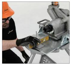
**4.** Level the tool from the top of the stand assembly, as shown above.
