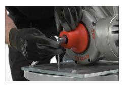
**3.** Loosen and remove the hex bolt and lock washer at the rear of the shaft, using a 5/16-inch socket.
