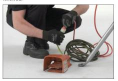
**2.** Plug the power drive cord into the safety foot switch, as shown above. Plug the safety foot switch cord into a grounded electrical outlet. Refer to the power drive manufacturer's operating manual for additional information.
