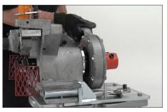
2. Align the square drive adapter of the Ridgid 700 power drive with the square drive of the tool head assembly, then push the power drive toward the tool head assembly, as shown above.
