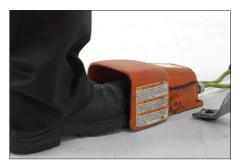
**3.** Depress the safety foot switch. Verify that the lower roll rotates away from the operator when viewed from the front of the tool. If the lower roll rotates toward the operator, see the appropriate power drive section for instructions to reverse rotation. Remove foot from the safety foot switch.
