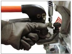
**4.** Rotate the hydraulic hand pump valve **counterclockwise** to open the valve and raise the upper roll to provide clearance for pipe insertion.
