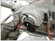
**1.** Using a  $\frac{3}{16}$ -inch hex key, loosen the set screw located on the top of the arm casting.
