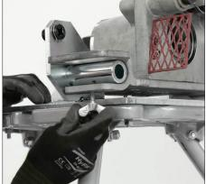
3. Tighten each wing head thumb screw to secure the tool head assembly onto the stand assembly. Ensure that the bolts are tightened evenly on both the left and right sides of the tool head assembly.
