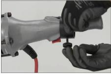
**7.** Install the trigger lock onto the power drive, as shown above. Tighten the mounting screw on the underside of the trigger lock.
