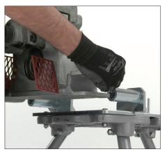
1. Using proper lifting techniques, lift the tool head assembly by the two handles with the roll guards facing toward you, as shown above. Do not lift the tool head by the roll guards.
