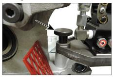
**2.** Tighten the thumbscrew to secure the hydraulic hand pump to the tool head assembly.
