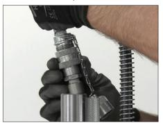
**4.** Remove the cap and install the quick-connect adapter onto the hydraulic cylinder connection, tightening completely. If the collar is not fully seated and tightened, the ball check may not operate properly, allowing hydraulic fluid to flow back through the hose.
