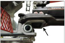
1. Place the hydraulic hand pump over one of the lifting handles on the tool head assembly, making sure that the lip on the underside of the pump's mounting plate aligns with the edge of the lifting handle.
