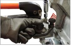
**21.** Rotate the hydraulic hand pump valve **counterclockwise** to open the valve and release the pipe from the tool.
