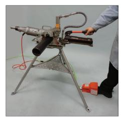
**16.** As the pipe rotates, begin the grooving process by pumping the handle of the hydraulic hand pump at a slow, steady rate. Ensure that the pipe remains against the lower-roll backstop flange. If the pipe does not remain against the lower-roll backstop flange, remove foot from the safety foot switch and re-position the pipe.
