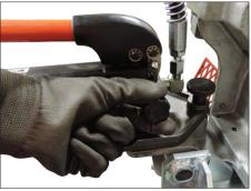
**9.** Rotate the hydraulic hand pump valve **clockwise** to close the valve.
