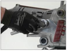
**4.** Using a %-inch square drive ratchet, tighten the mounting screw to secure the Ridgid 700 power drive to the stand assembly.
