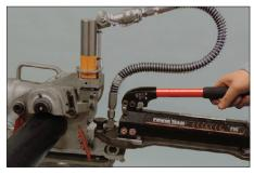
**10a.** While supporting the pipe, pump the handle of the hydraulic hand pump to place the upper roll into light contact with the pipe.
