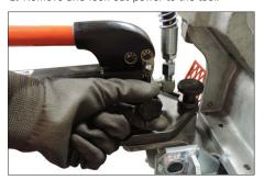
**2.** Raise the upper roll arm to its maximum position by rotating the hydraulic hand pump valve **counterclockwise** to open the valve.
