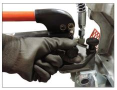
**3.** Confirm that the hydraulic hand pump valve is not holding any residual pressure by rotating the hydraulic hand pump valve **counterclockwise** to open the valve.
