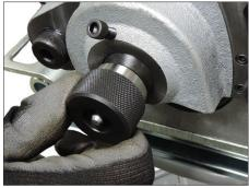
**3.** Insert the upper shaft into the arm casting and upper roll.
