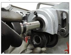
**2.** Position the upper roll in the pocket of the arm casting.
