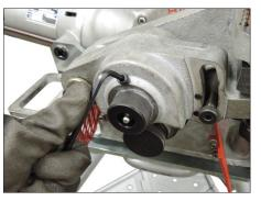
**4.** Using a 3/6-inch hex key, tighten the set screw to secure the upper shaft in position. Ensure that the upper roll rotates freely.
