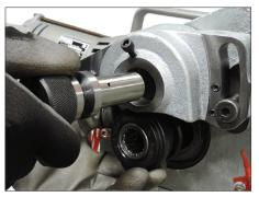
**3.** Remove the upper roll. Store the upper roll in the provided tool bag to prevent damage.
