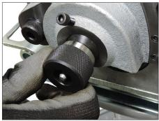
**2.** Prepare to support the upper roll while sliding the upper shaft out of the arm casting.
