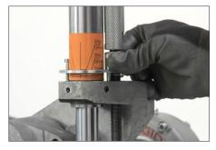
**13.** Turn the travel stop to adjust the height of the depth stop indicator top plate.
