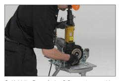
2. Hold the Rems Amigo 2 Compact power drive with the motor handle facing upwards. Align the drive bushing of the tool head assembly with the retaining ring of the power drive. Push the power drive over the drive bushing.
