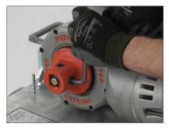
**5.** Using a %-inch hex key, tighten each set screw on the square drive adapter of the Ridgid 700 power drive.
