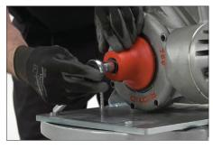
**5.** Install and tighten the hex bolt and lock washer at the rear of the shaft, using a \%-inch socket.
