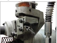
2. Apply grease under the pivot block.
