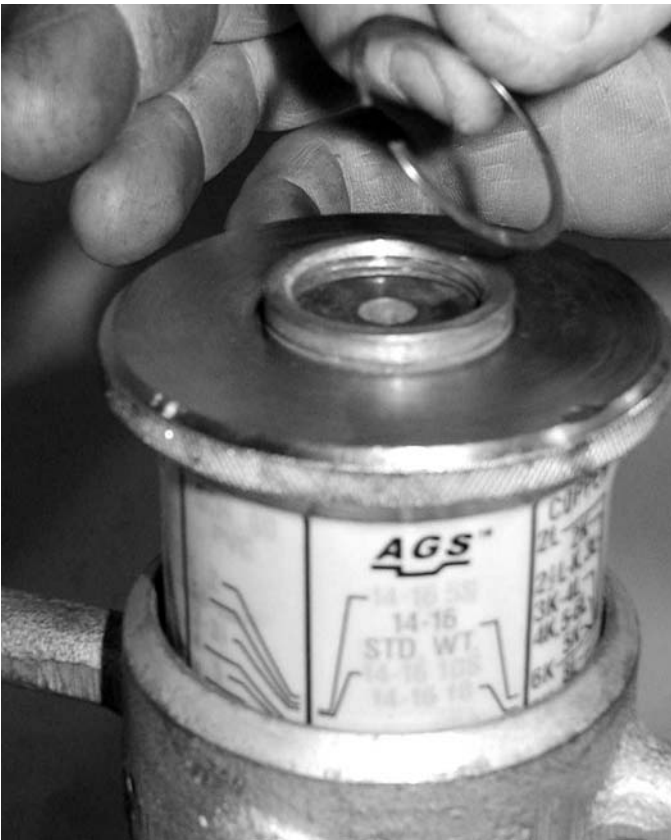
26. Re-install the retaining ring on top of the barrel.
