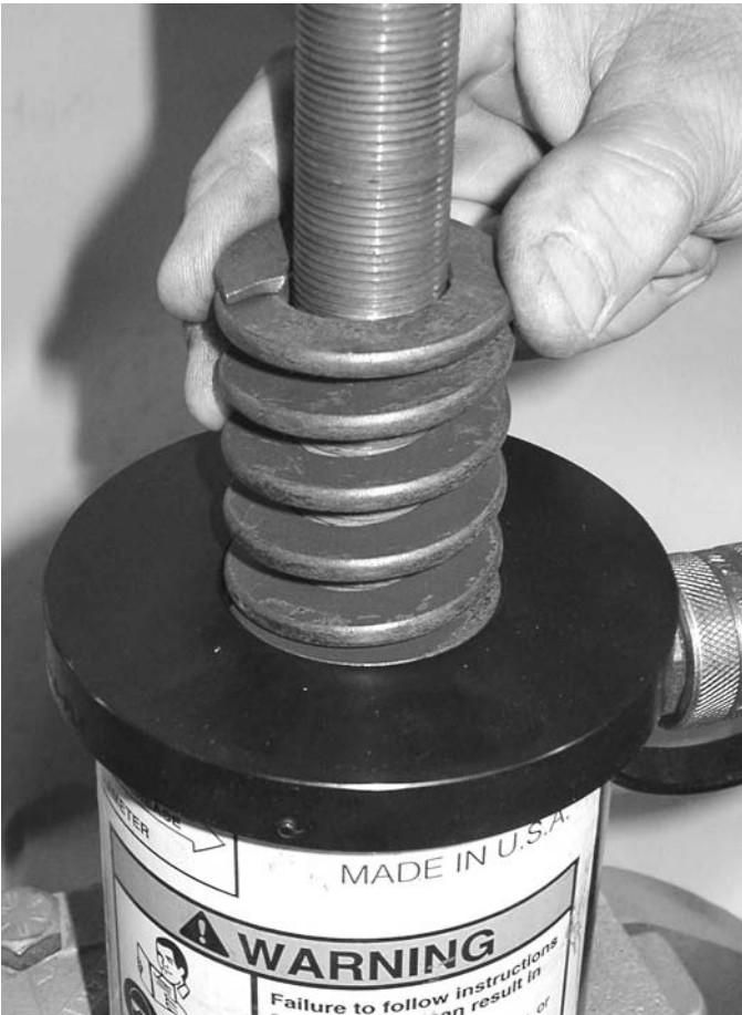
10. Slide the new upper roll retract spring down onto the tool's threaded rod. Seat the spring in the new return spring seat recess.
