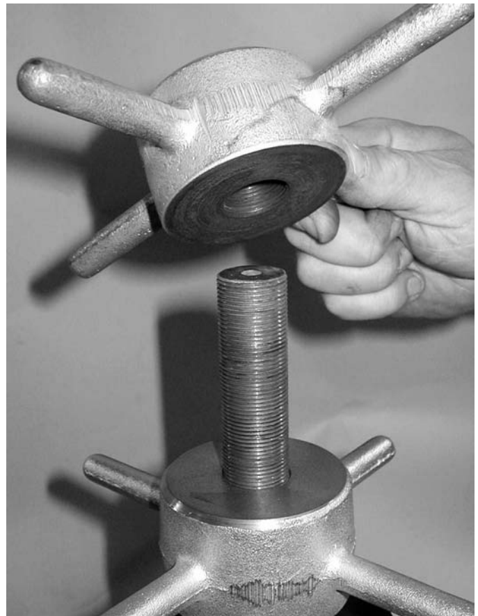
13. Re-install the depth adjuster by threading clockwise onto the tool's threaded rod. Continue to rotate this adjuster until it seats against the adjuster lock installed in Step 12.
