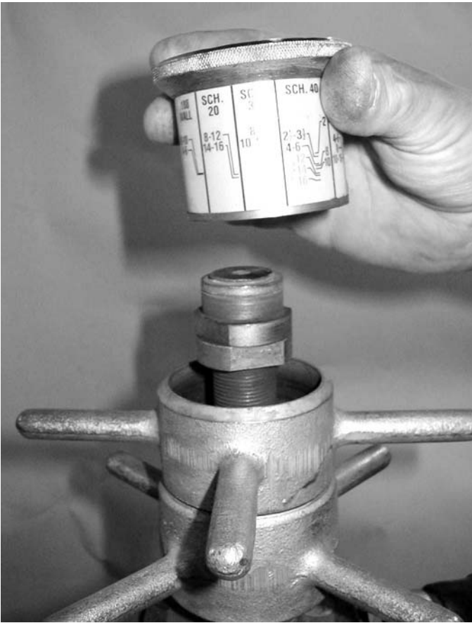
25. Re-install the depth adjuster barrel.
