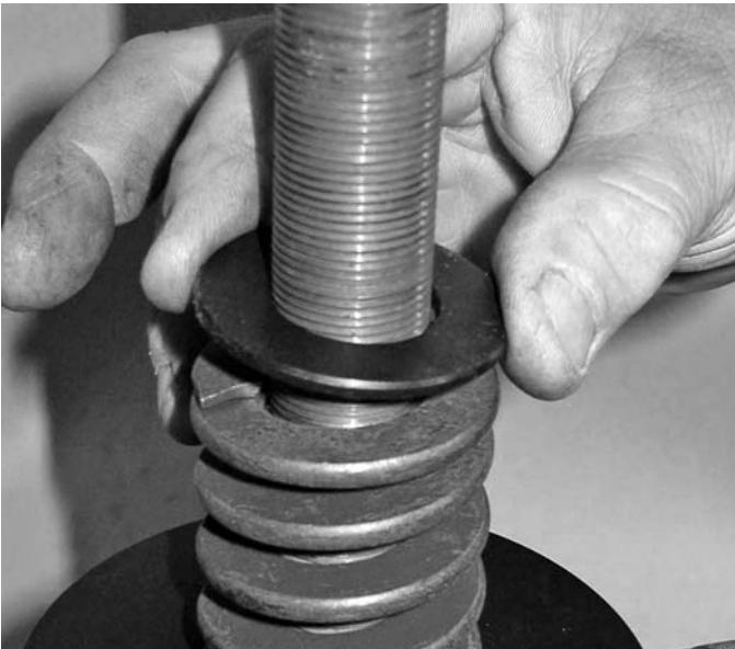
11. Install the new spring washer by sliding the washer down onto the tool's threaded rod and placing the washer on top of the new compression spring.
