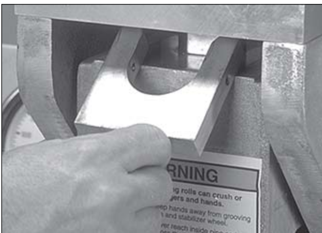
8. Remove the slide spacer by snapping it out directly, as shown above.
