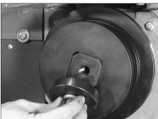
4. Install the lower-roll washer and lower-roll retaining bolt.
