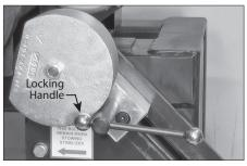
1. Loosen the locking handle of the pipe stabilizer.
