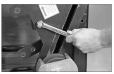
**4.** Remove the lower bolt and lock washer from the pipe stabilizer assembly. Keep this bolt and lock washer for re-installation. If necessary, loosen but do not remove the upper bolt.
