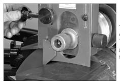
**7.** Loosen the knob on the side of the roll guards to drop the sliding guard onto the guard setting pad. Tighten the knob.
