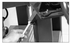
**7.** Raise the hand pump to the operating position. Insert the leg of the hand pump assembly into the bracket on the tool.
