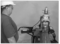
**6.** The operator shall be positioned, as shown to the left. Pump the handle of the hand pump until the upper roll moves down and comes into firm contact with the pipe. Remove hands from the pipe.
