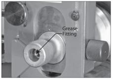
**4.** Lubricate the upper roll bearings every time rolls are changed and after every 8 hours of operation. A grease fitting is provided on the front of the upper shaft, as shown to the left. Refer to the "Maintenance" section for additional information.
