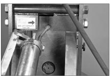
**2.** Grease the slide gibs. The slide gib grease fitting is located on the back of the slide.
