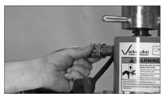
**10.** Remove the cap from the power cylinder. Connect the hydraulic hose from the hand pump to the power cylinder using the quick connections provided.
