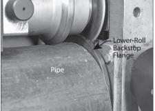
**6.** Open the hand pump valve by turning it counterclockwise. This will allow the upper roll to move to its highest position.
