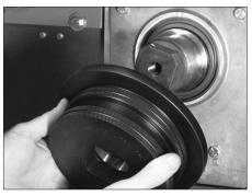
**3.** Align the square end of the main shaft with the square hole in the lower roll. Push the lower roll completely onto the main shaft. Verify that the markings on the lower roll are facing out.
