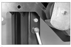
**6.** Remove the two bolts and two lock washers from the bag located in the larger storage box. Install the bolts with lock washers into the holes in the pipe stabilizer and tool frame. Tighten the bolts until the lock washers become flattened.
