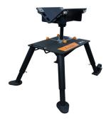
The Victaulic VAPS112 Pipe Stand is a portable, adjustable, roller-type pipe stand that contains four legs for additional stability. The VAPS112 supports pipe sizes ¾ to 12 inches/DN20 to DN300 (1½-foot/0.5-meter to full, single 20-foot/6-meter random lengths) and has a load rating of 1075 pounds/490 kilograms. The turnstile design permits ease of grooving for both pipe ends. Contact Victaulic for details.
