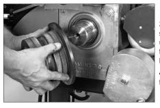
**3.** Remove the lower roll by pulling it off the main shaft. If the lower roll cannot be removed by hand, use a conventional gear puller. Be careful not to lose the Woodruff key located in the main shaft. Store the lower roll in the larger storage box.
