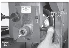
**2.** Pull the upper shaft locking pin out of the slide until it stops.
