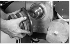
**3.** Align the keyway in the lower roll with the Woodruff key inserted in the main shaft. Verify that the markings on the lower roll face outward.
