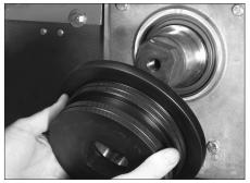
**3.** Remove the lower roll by pulling it off the main shaft. If the lower roll cannot be removed by hand, gently tap around the circular face of the lower roll to loosen it. Store the lower roll in the larger storage box.
