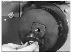
**2.** Remove the lower-roll retaining bolt and the lower-roll washer.
