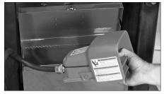
11. Remove the safety foot switch from the storage box. Place the safety foot switch in a location that provides ease of access for the operator. DO NOT ATTEMPT TO OPERATE THE TOOL WITHOUT A SAFETY FOOT SWITCH.
