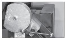
**4.** Grease the stabilizer wheel. A grease fitting is accessible from the rear side of the wheel guard. The stabilizer wheel may need to be rotated to gain access to the grease fitting.
