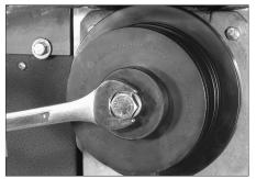
**1.** Using an adjustable wrench, loosen the lower-roll retaining bolt.
