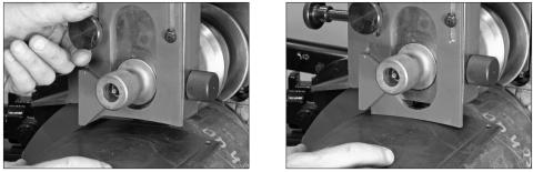
**6.** Hold the correct guard setting pad firmly against the pipe and push it under the roll guards. Loosen the knob on the front of the roll guards to drop the plate onto the guard setting pad. Tighten the knob.
