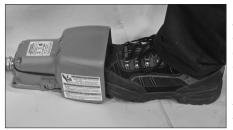
**7.** Depress and hold down the safety foot switch. This will produce clockwise rotation of the lower roll when viewed from the front of the tool. Check the tracking of the pipe as it rotates to verify that it remains in contact with the lower-roll backstop flange. If the pipe does not remain in contact with the lower-roll backstop flange, stop the tool by releasing the safety foot switch. When the pipe stops rotating, verify that the pipe is positioned properly on the lower roll.
