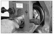
**2.** Install the proper upper roll behind the slide, as shown to the left. Verify that the markings on the upper roll are facing forward. While supporting the upper roll, insert the upper shaft into the slide and upper roll.
