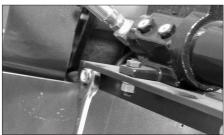
**9.** Tighten the nut located on the back side of the hand pump assembly.
