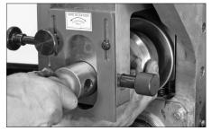
**3.** While supporting the upper roll, remove the upper shaft from the upper roll/slide by pulling it straight out.
