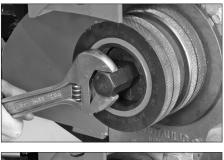
**1.** Using an adjustable wrench, loosen and remove the lower-roll retaining bolt.
