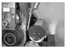
**3.** Grease the main shaft bearings through the fitting located on the side of the tool.
