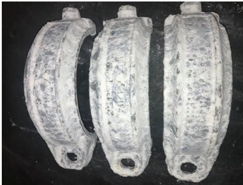
Figure 3: Mechanically Deposited Zinc Coating Post-Test
