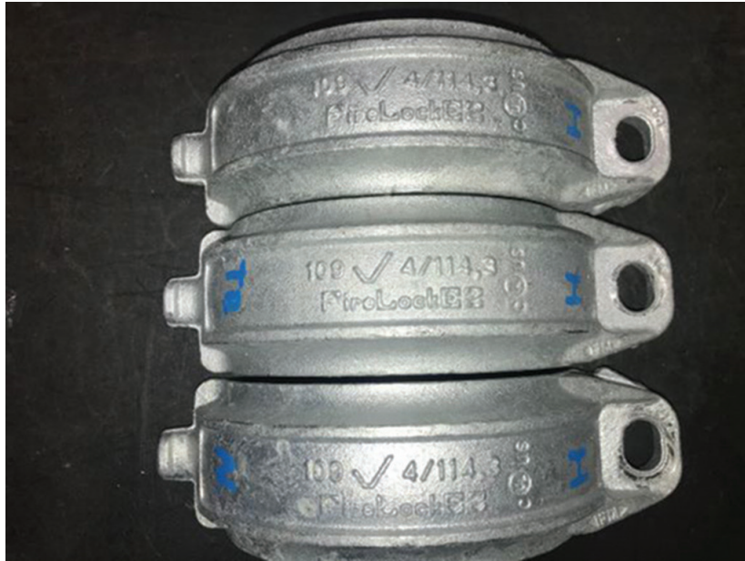
Figure 2: Hot Dip Galvanized Pre-Test
