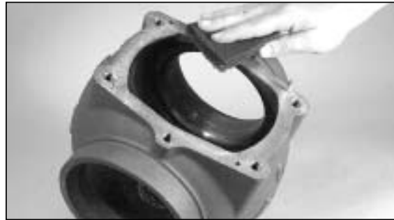
12. Clean the mounting surface of the valve's body with a mild-abrasive pad.
