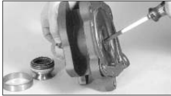
10. Remove the packing gland and the packing set from the bonnet. Use a screwdriver to pry the items from the bottom side of the bonnet.
