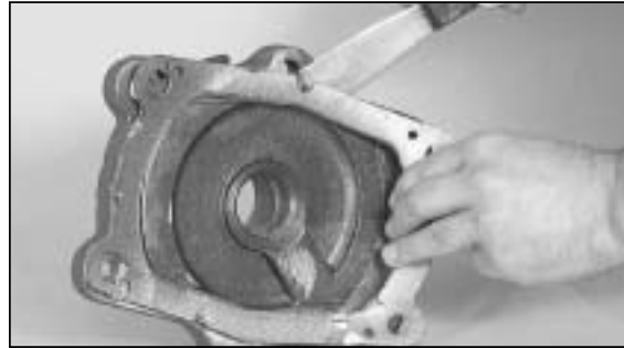
11. Remove the gasket by using a putty knife. 11a. Clean off any excess residue with a mild-abrasive pad.
