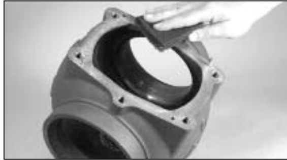
9. Clean the mounting surface of the valve's body with a mild-abrasive pad.
