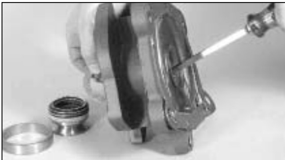
7. Remove the packing gland and the packing set from the bonnet. Use a screwdriver to pry the items from the bottom side of the bonnet.
