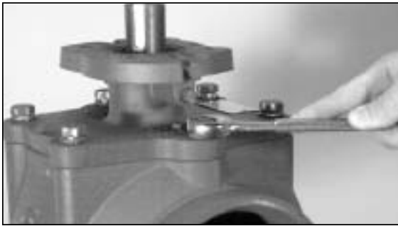
8. Remove the six bolts from the valve's body.
