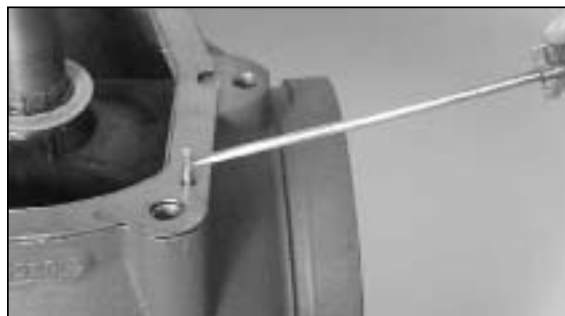
11. Align the bonnet with the dowel pins.
