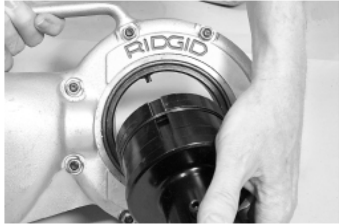
10. Install power drive adapter into power drive by aligning the drive tangs (shown in Step 7) with the recesses in the adapter (shown in Step 8). Make sure the shaft of the adapter (shown in Step 8) faces the same side of the power drive as the tapped hole (shown in Step 9).
