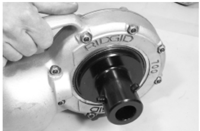
10a. Make sure the power drive adapter engages completely into the power drive, as shown above.
