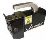
Includes base lathe adapter cutting head, full set of tool bit holders (1 each), and complete set of tool bits (10 each) for cut grooving 3-36'' cast and ductile iron pipe, all included in a weather and impact resistant carrying case.
