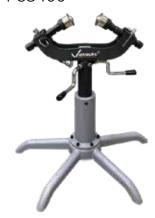
Adjustable Pipe Stands are portable and self-standing units. Rotating design allows pipe to be spun around for grooving of both pipe ends without removing pipe from the stand. They are designed for direct use with roll grooving tools: RG3212 and RG3400.
