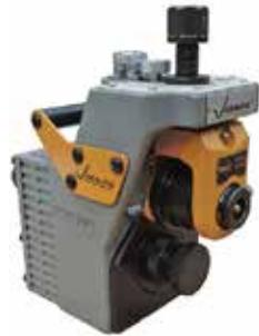
The RG2300 is a combo roll grooving tool that can be used manually in-air or mounted to a power drive for increased productivity. This tool provides 1 to 12 inches of grooving capacity in a compact, lightweight package well suited for field use. The available tool configurations are listed below.
