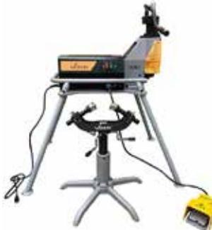
The RG3400 is a self-contained, transportable roll grooving tool with an integral drive motor and hydraulic feed unit. The RG3400 requires a 120V, 15-amp or 220V, 8-amp power source and is supplied with a pipe stand for 1 – 12" pipe. The available configurations for this tool are listed below.
