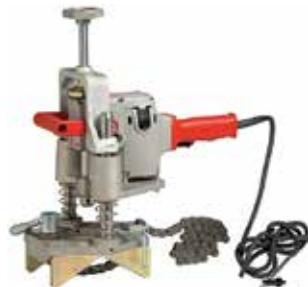
Includes three-piece hole cutting tool (Base, drill motor and feed assembly), arbor assembly, coupon remover, 2 pilot drills with coupon retaining springs and operating instructions. Requires grounded 120/1/60 – 10 amp electrical supply. (220/1/60 – 10 amp no cost option). For sizes over 2 3/4"/70 mm or when speed control is needed for various materials, use an inline speed controller to reduce hole saw wear and improve performance.
