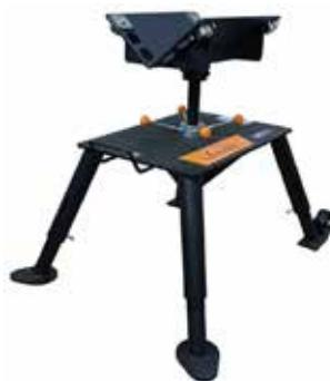
Adjustable Pipe Stands are portable and self-standing units. Turnstile design allows pipe to be spun around for grooving of both pipe ends without dismounting pipe from stand. Unique trough design allows for rotational and forward/traverse movement. They are designed for direct use with roll grooving tools: VE272SFS, VE268, VE270FSD.
