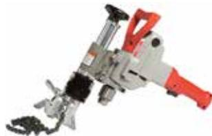
The HCT908 Hole Cutting Tool is a one-piece tool designed to cut holes up to 2 3/4" carbon and stainless steel pipe. This allows for use of **Mechanical-T**, Strapless Outlet, Thermometer Outlet and Style 922 Outlet Tee. Requires 110 volt power supply to operate. For sizes over 2 3/4"/70 mm or when speed control is needed for various materials, use the supplied inline speed controller to reduce hole saw wear and improve performance.
