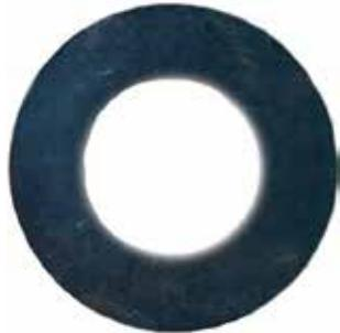
Victaulic flange adapters require a smooth, hard surface at the mating flange face for effective sealing. Some applications, for which the Victaulic flange adapter is otherwise well suited, do not provide an adequate mating surface. In such cases, it is recommended that a metal flange washer be inserted between the Victaulic flange adapter and the mating flange to provide the necessary sealing surface. See Spare Parts Section for flange washer prices.
